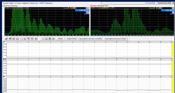
**Real-Time View:** The software displays the A-Scan and B-Scan data in real-time during the scan.
